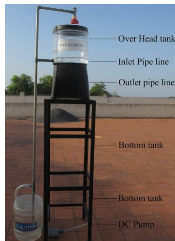
Figure 7. Water pumping system setup with vertical storage assembly.
